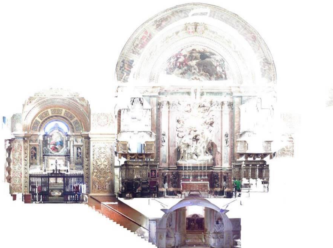
Figure 10: Detailed sections through the Crypt produced using a 3D scan, showing the oculi and the Main Altar
